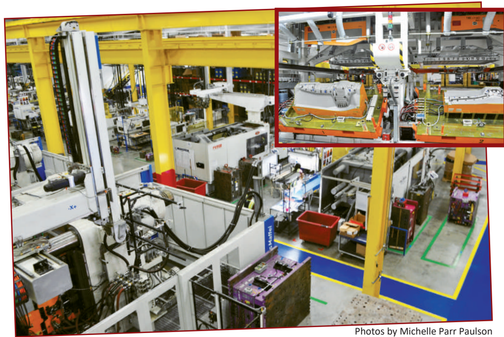
IAC's Anniston plant, above, has 36 injection molding machines and a dual-platen vacuum forming line, inset.
